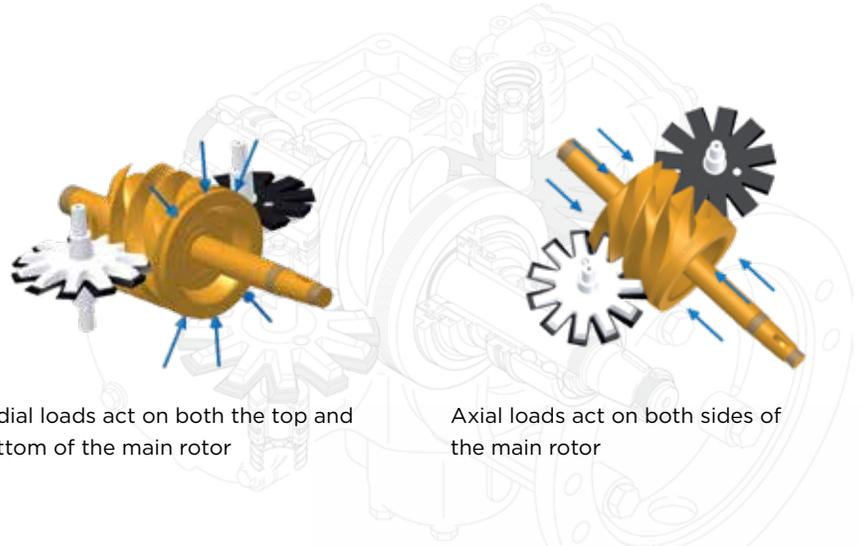
Radial loads act on both the top and bottom of the main rotor
